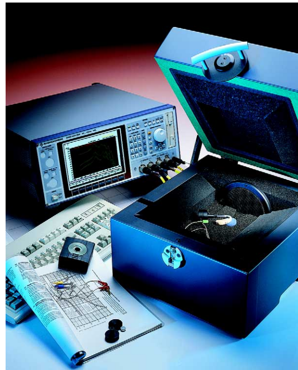
Test setup with acoustic test chamber (photo 43159)
