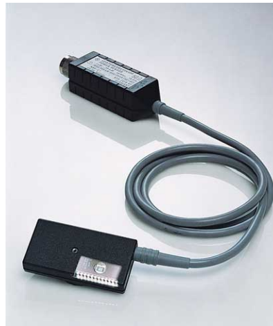
Calibration data for each sensor are stored in an EPROM in the sensor's connector (photo 37902)
