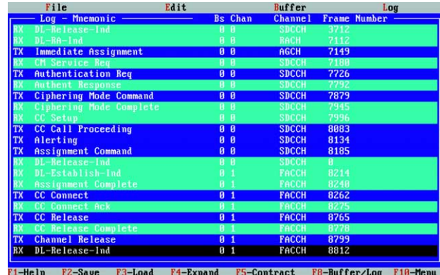
Display of message sequence at layer 3 level
