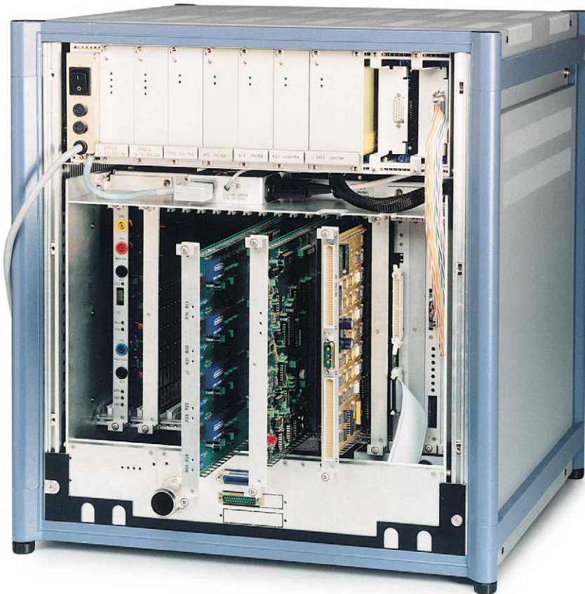
Stimulus and measurement modules are inserted into the rear of TSA (photo 38860)
