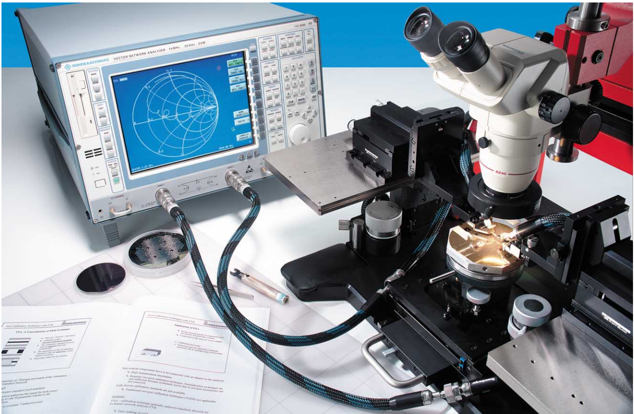
The Rohde&Schwarz calibration techniques offer maximum convenience and accuracy also for on-wafer measurements (Vector Network Analyzer ZVM, photo 43453-6)
